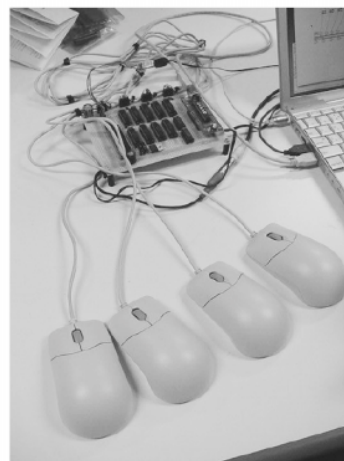
Figure 4. 4 * PS2 Mouse, Video out, GAINER I/F system.
