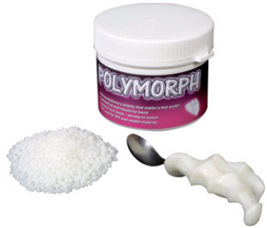
Figure 5. Polymorph (Polycaprolactone) material, also known as “Shapelock” or “Friendly Plastic”, will be used to sculpt the shape of the right-hand controller around the completed electronics for The Fingers.
