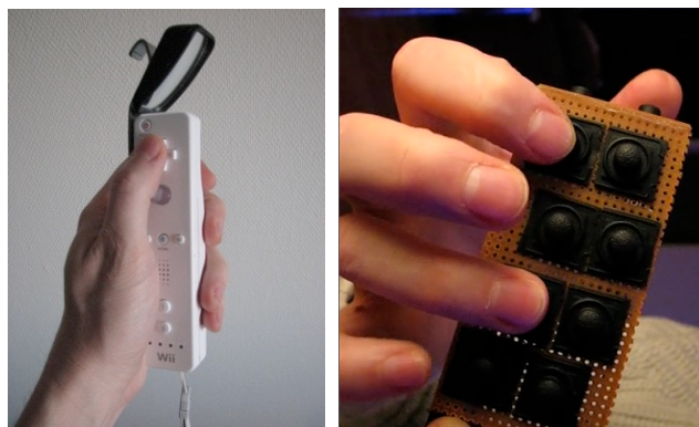
Figure 1. The Fingers: a performer uses the Nintendo Wiimote with a periscope-style mirror in their left hand, while the right hand uses a custom CREATE USB Interface (CUI)-based expression controller.
